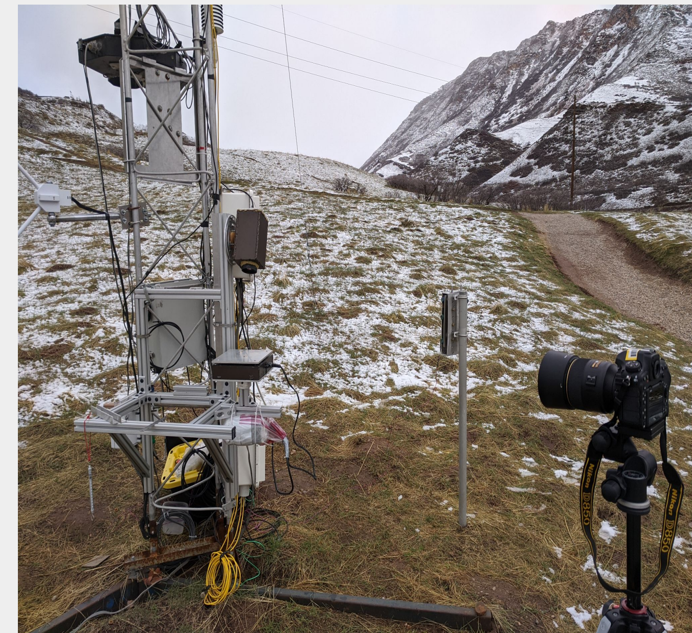
Instruments set up at Alta Ski Area, including the Snow Pixel, the DEID, the MASC, and instruments to measure environmental conditions.
