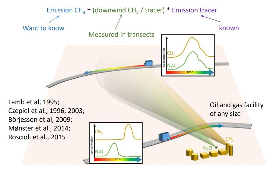
Early, this work employed one tracer,  $N_2O$  we took single cylinder of aux. tracer  $C_2H_2$
