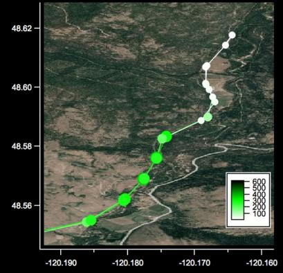
Mobile ground measurements resolve substantial changes in atmospheric composition
