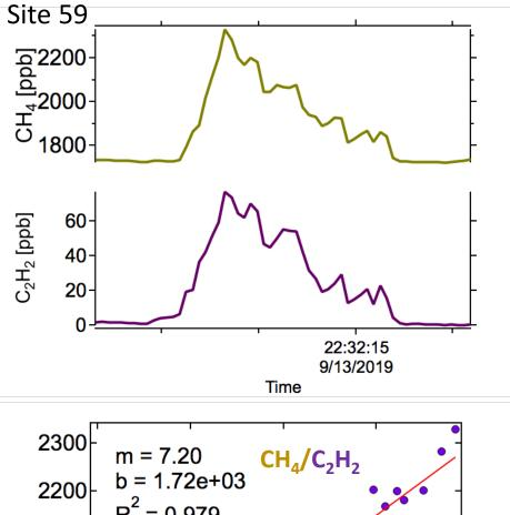
Method to quantify: tracers flux ratio
