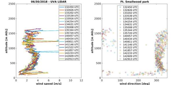
Wind profiles from about 100 m to ~3000 m or more (depending on atmospheric conditions and lidar settings) at ~1 km horizontal spacing and 30 m vertical spacing.
